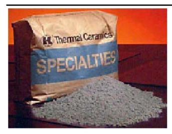
Moral Coolcast 100 LW – K is a lightweight insulating castable based on selected lightweight aggregates and high purity calcium aluminate cement. It has a temperature rating of 1100°C and can be either cast or gunned.
