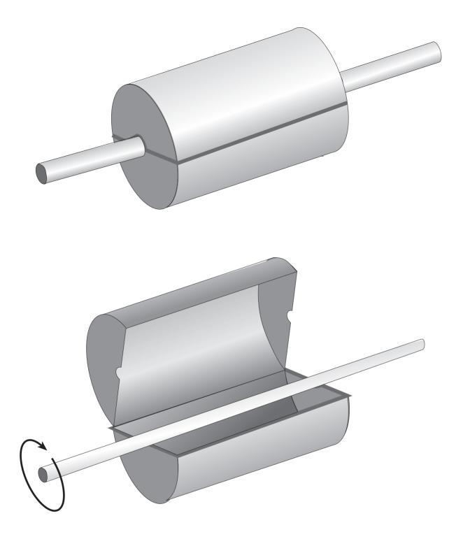
Planned manufacture of a 250mm diameter x 500mm long cylinder made from a fine woven stainless steel wire quite open, similar to open flyscreen. It is hinged in two with quick release clasps for quick and easy emptying. Set up on a spindle shaft, driven like a rotisery with a variable speed windscreen wiper motor. The ends supported on steel supports. The ends of the cylinder are also made of the same fine stainless woven wire, which will allow viewing of the roasting beans.
