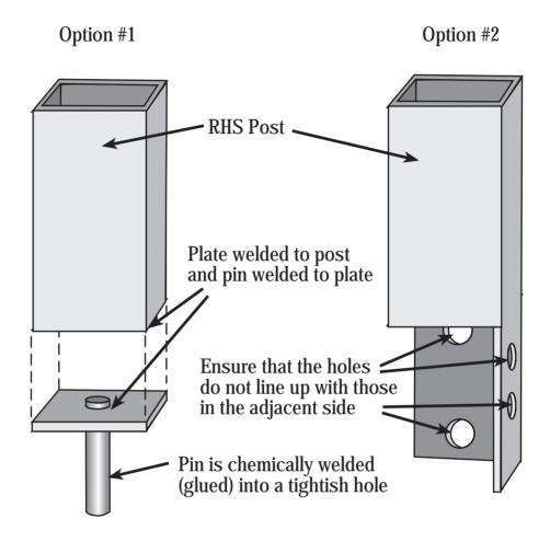
Note: The pin can be welded in a corner of the plate (rather than in it's centre), making the hole furtherest infrom the cement slab
