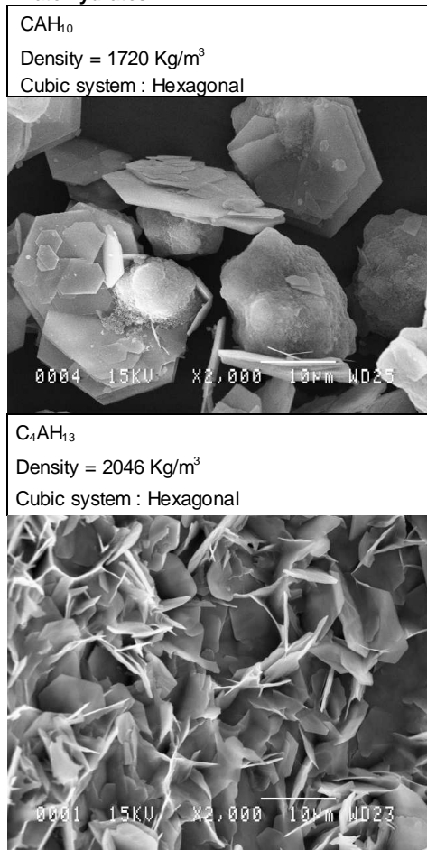
Fig. 1: Key properties and Micrographs of the calcium aluminate hydrates
