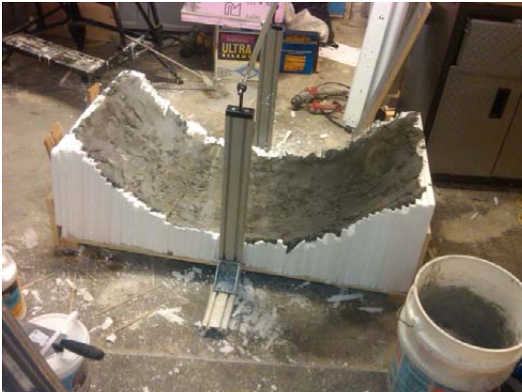
Made a jig to cast Glass Fiber Reinforced Concrete (GFRP) shells; I knew I would be covering the Insulfrax in the winter and wanted a fast way to get a hard, weather resistant shell.
