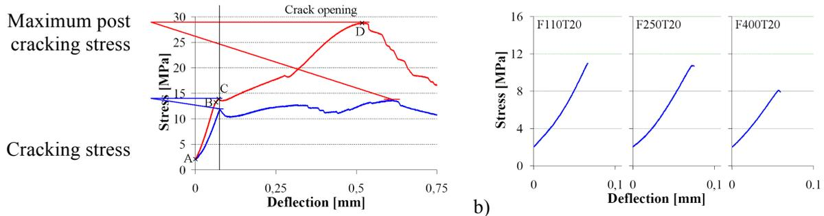
**Figure 2.** Four points bending behaviour curves (stress vs. deflection): (a) for HF05 (blue) and HF20 (red) grades dried at 110°C and tested at room temperature, (b) for the NF HF20 grade (unreinforced material) fired at different temperature and tested at room temperature.
