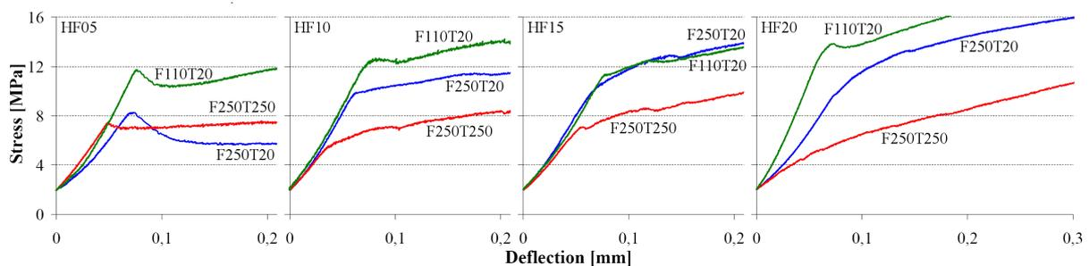
**Figure 3.** Stress-deflection curves in four points bending of steel fibre reinforced concretes fired at 110°C and tested at 20°C (green), fired at 250°C and tested at room temperature (blue), fired at 250°C and tested at 250°C (red) for the HF05, HF10, HF15 and HF20 grades
