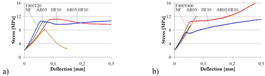
**Figure 6.** Stress-deflection curves in four points bending of NF (green), HF10 (blue), AR05 (orange) and AR05-HF10 (red) grades fired at 400°C and tested at room temperature (a) and at 400°C (b)
