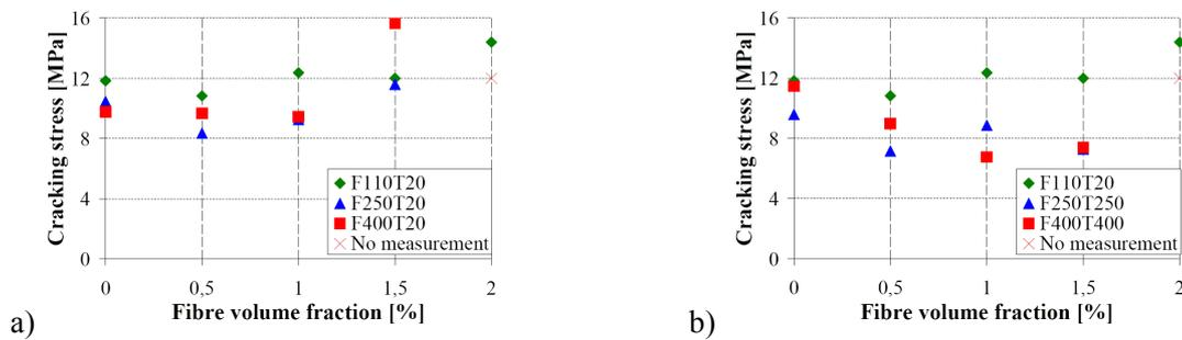
**Figure 9.** Cracking stress in four points bending of steel fibre reinforced concretes fired at 110°C (green points), 250°C (blue points) and 400°C (red points) and tested at room temperature (a), and at the firing temperature (b)
