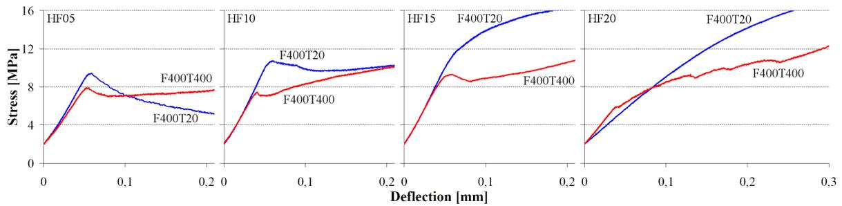
**Figure 4.** Stress-deflection curves in four points bending of steel fibre reinforced concretes fired at 400°C and tested at room temperature (blue) and fired at 400°C and tested at 400°C (red) for the HF05, HF10, HF15 and HF20 grades
