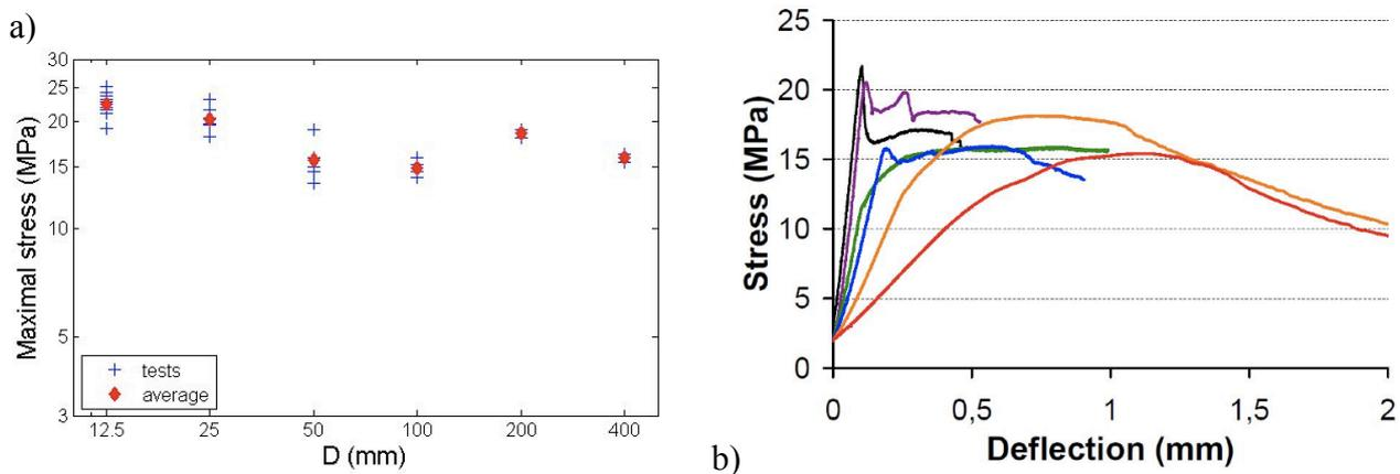
**Figure 8.** Results of size effect sensitivity results for a metallic fibre reinforced refractory concrete tested in 3 points bending ( $V_f=1,5\%$ ), (a) Maximal stress (b) Behaviour curves.
