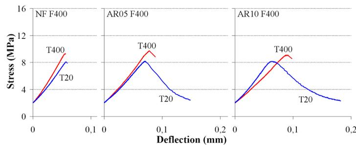
**Figure 5.** Stress-deflection curves in four points bending for NF, AR05 and AR10 grades fired at 400°C and tested at room temperature.
