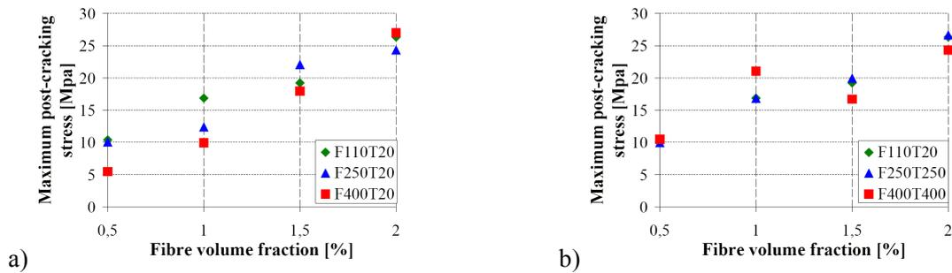
Figure 10. Maximum post cracking stress  $s$  in four points bending of steel fibre reinforced concretes fired at 110°C (green), 250°C (blue) and 400°C (red) and tested at room temperature (a), and at the firing temperature (b).
