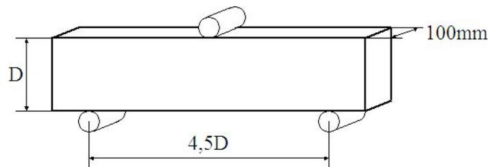
**Figure 1.** Three points bending geometry of samples considered to study the size effect sensitivity.
