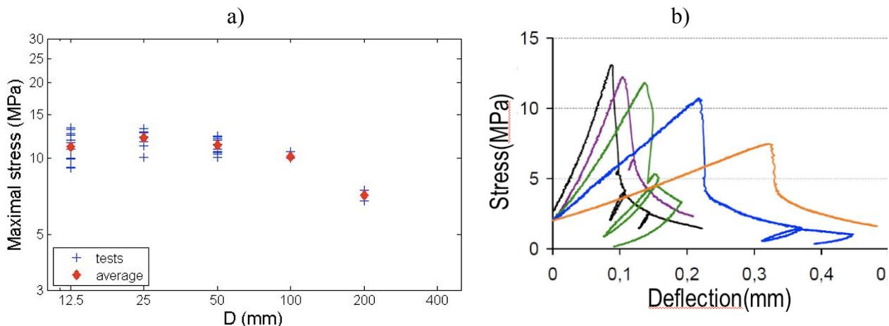
**Figure 7.** Results of size effect sensitivity results for unreinforced refractory concrete tested in 3 points bending, (a) Maximal stress (b) Behaviour curves.
